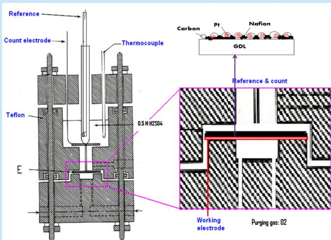
Fig. 1. The scheme of the Teflon half-cell
