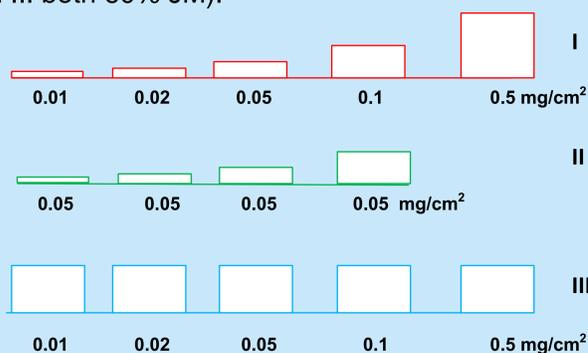
Fig. 2. The scheme of the types of electrodes with different thickness and platinum loading, mg/cm<sup>2</sup> as indicated by arabic numbers.
